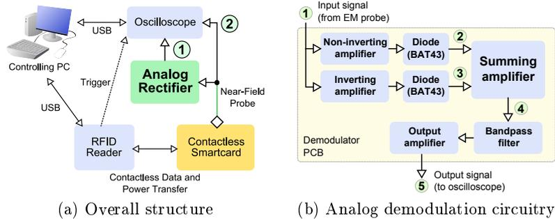
Fig. 1: Measurement setup
