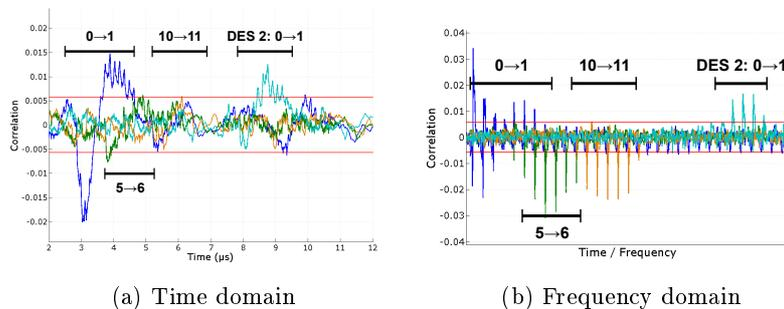
Fig. 5: Correlation coefficients for the Hamming distances between rounds of the 3DES, 500,000 traces
