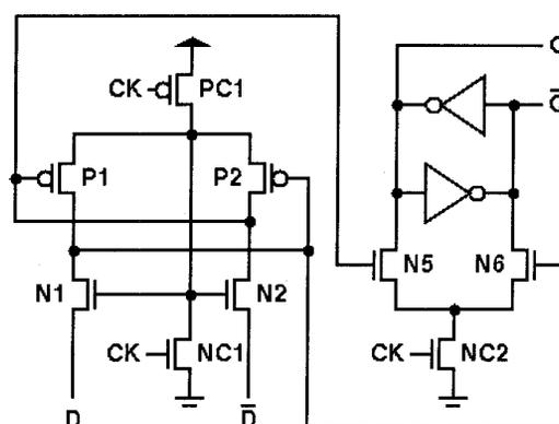
Figure 2. New CVSL Flip-flop.
