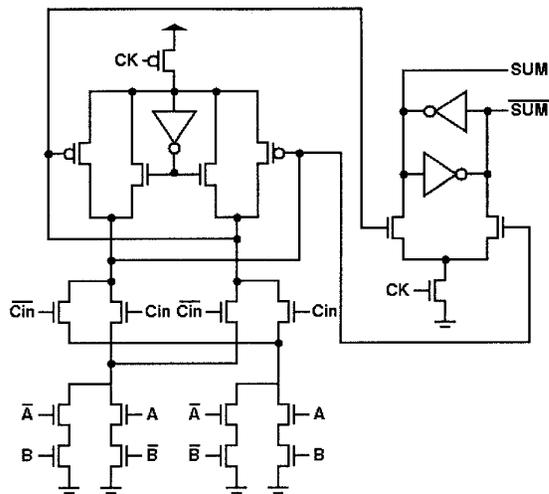
**Figure 3.** Add-and-Delay Circuit using the New CVSL Flip-flop and DCVSPG technique
