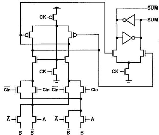
**Figure 4.** Add-and-Delay Circuit using the Yuan and Svensson's CVSL Flip-flop.
