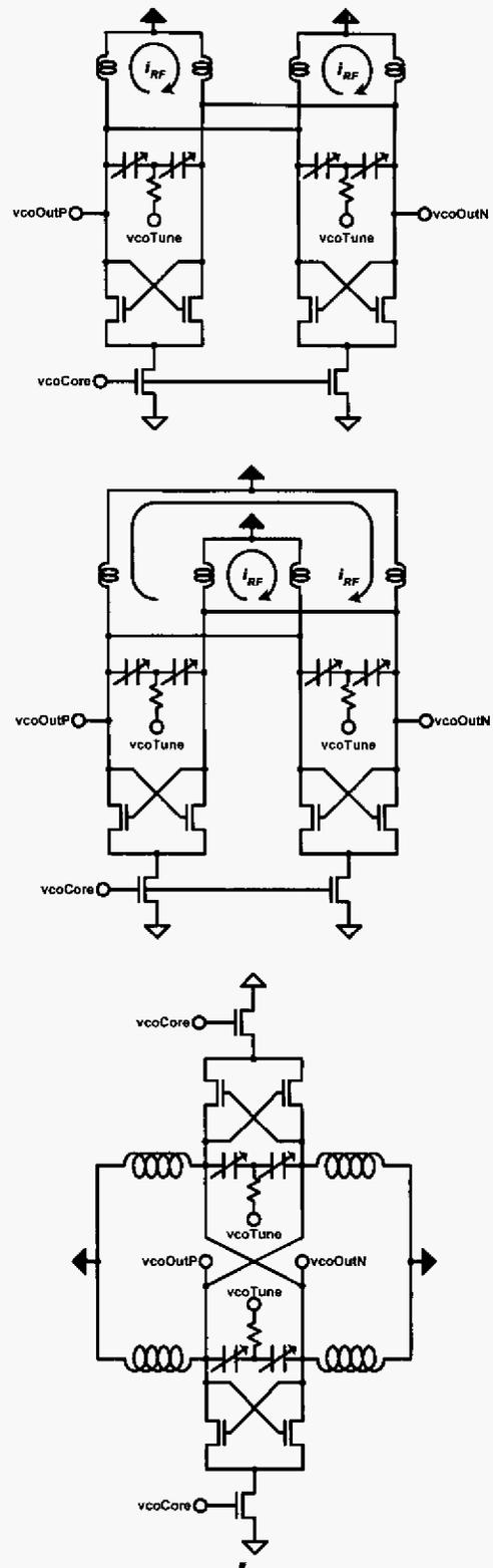
Fig. 2. Circular-geometry oscillator evolution: The initial two parallel-connected VCOs are finally arranged to form a balance-scale shaped circular-geometry VCO.
