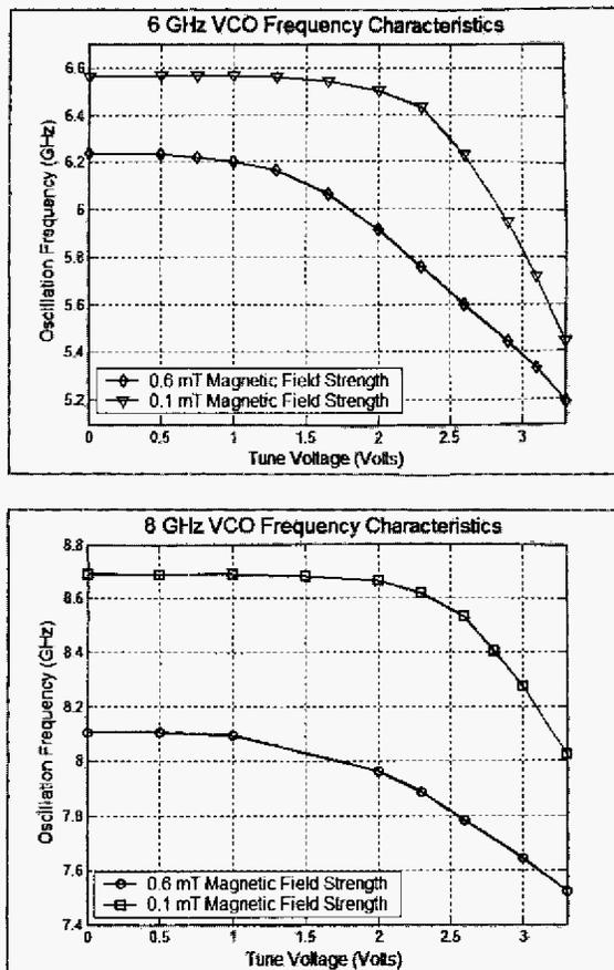
Fig. 5. Frequency characteristics for the 6 GHz (top) and 8 GHz (bottom) VCOs.
