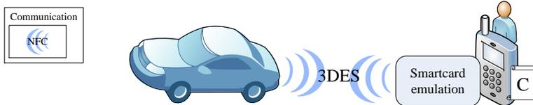
Fig. 4: For executing the granted rights at an NFC object, the smartphone emulates a contactless cryptographic smartcard (here, a Mifare DESFire card). The NFC reader in the door lock of the car detects the presence of the smartphone and initiates the communication. After establishing a secure channel (with 3DES), the credential **C** is transferred from the phone to the car.
